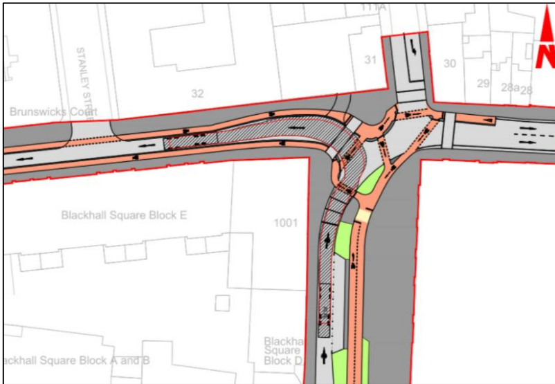
Figure 4.118.1: Swept-path of Rigid HGV turning from George's Lane into Brunswick Street North
