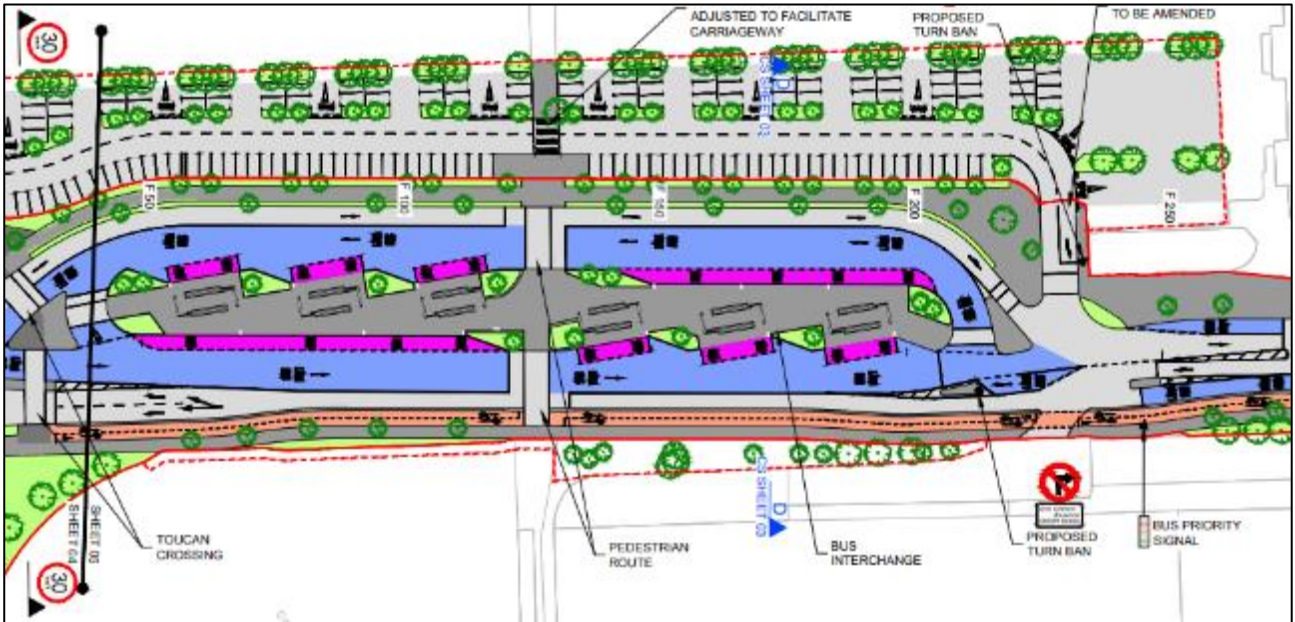
Figure 2.9.29: Bus Interchange Layout
