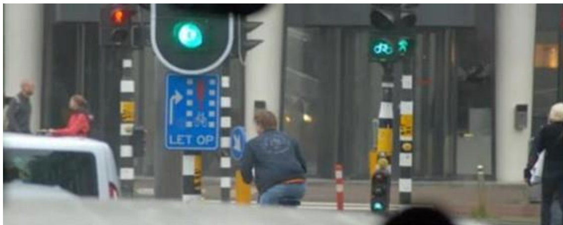
Figure 2.9.10: Example from the Netherlands of traffic signals + give way signage controlling turning traffic and cyclists (Source: Dutch Design Guide Ontwerpwijzer Fietsverkeer)
